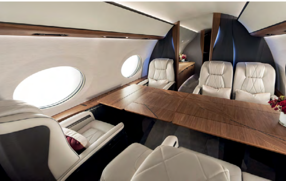
MSB stress tests its tables for more 20,000 open-close cycles and forces of 9G. Photo: MSB
