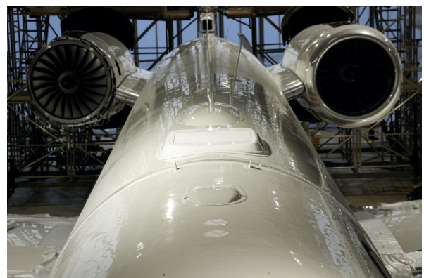
Starlink top mounted fuselage antenna installation
